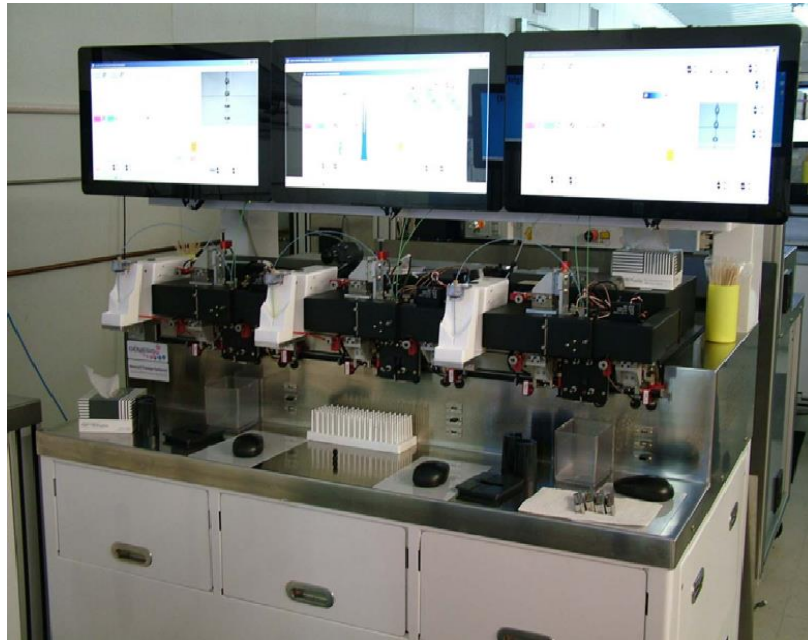
Figure 6: Genesis III™ cytometer for sperm sexing (42)
